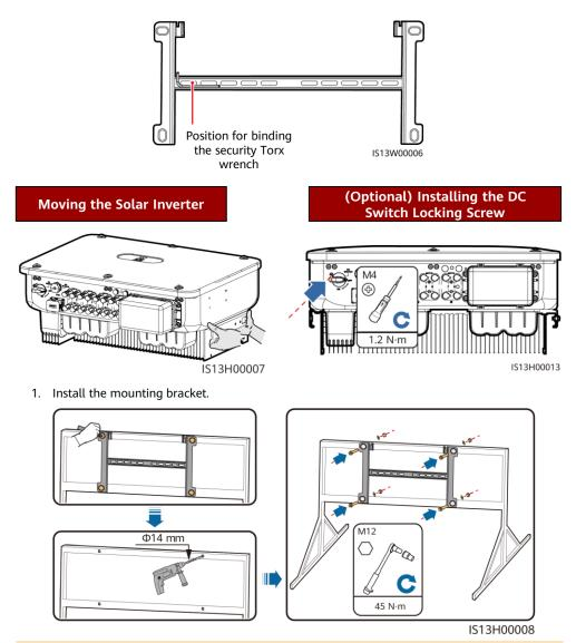
It is recommended that anti-rust measures be taken on the positions for drilling holes.
