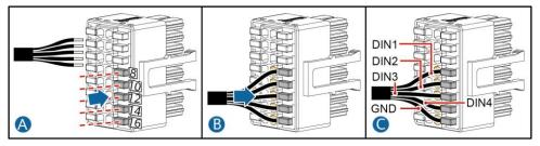
• Connect the rapid shutdown signal cable.
