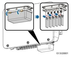
2. Connect the AC output power cable (using a five-core cable as an example).
