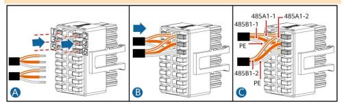
• Connect the RS485 communications cable to the power meter.
