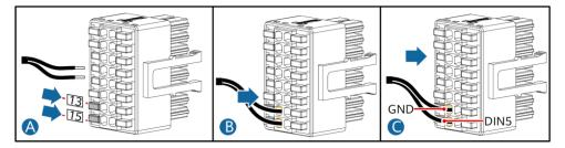
2. Connect the signal cable connector to the communications port.
